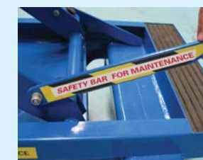
Maintenance Safety Bar
